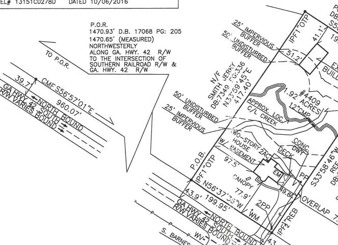
POINT OF BEGINNING POINT OF REFERENCE P.O.R. GAS MARKER/GAS METER OPEN TOP PIPE IRON PIN FOUND IRON PIN SET 1/2" FEBAR W/ CAP C/G P/L R/W L.L.L. CURB AND GUTTER PROPERTY LINE RIGHT-OF-WAY LAND LOT LINE CMF CONCRETE MONUMENT FOUND POINT ON LINE B.O.C. FNC EP PC BACK OF CURB FENCE CORNER EDGE OF PAVEMENT PROPERTY CORNER OLP ØPP LIGHT POLE POWER POLE GUY WIRE EXISTING JUNCTION BOX
