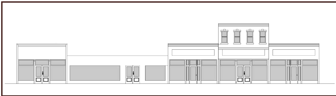
Inappropriate horizontal structure. Avoid buildings that appear to be too wide compared to the surrounding context. Front view.
