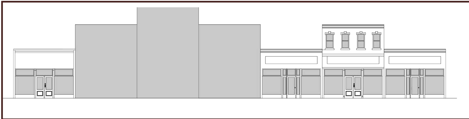
By segmenting the facade, larger buildings can be designed to fit in with the historic context of the existing buildings. Front view.
