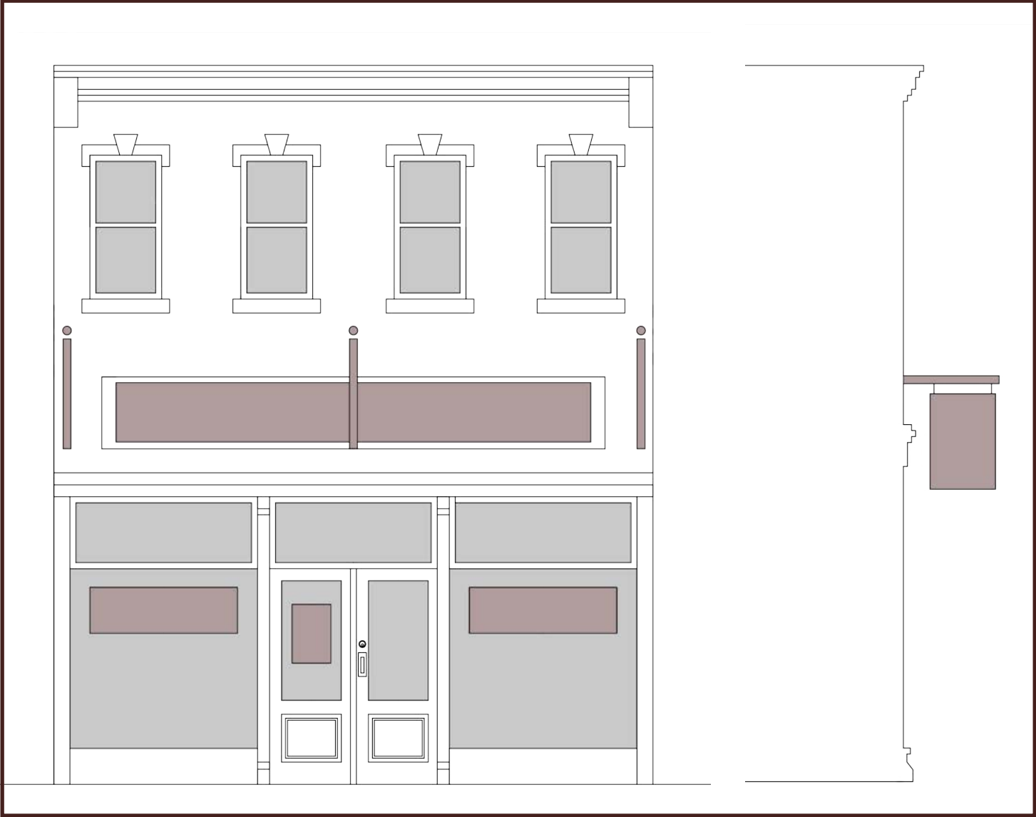
Traditional Sign Locations. Front view.
