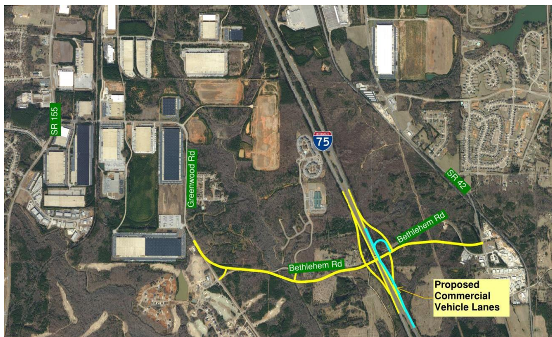
Figure 3.8: Interchange Alternative 4A
