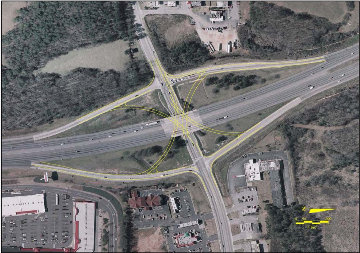
Figure 7.1 : Build Alternative 1 – Single Point Urban Interchange (SPUI)
