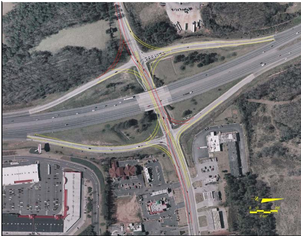
Figure 7.2 : Build Alternative 2 – Diverging Diamond Interchange (DDI)
