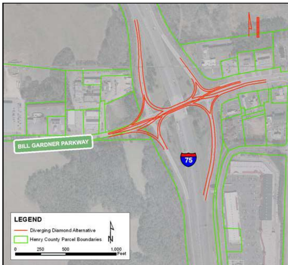
Figure 8.4: Right-of-Way Requirements – Diverging Diamond Interchange
